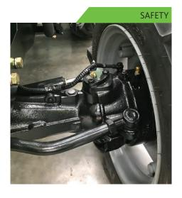
The Deutz-Fahr 4E series is fitted with 4 wheel wet disc brakes as a standard. This systems works with wet disc brakes fitted not only on rear axle but the front axle resulting in all 4 individual wheels having braking power.
